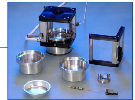
temperature control unit TEC 250/DCAT with accessories
